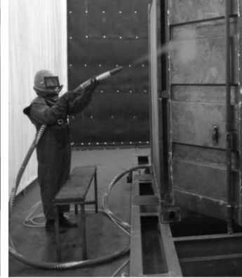
Grit blasting in the workshop takes place in "chamber" to reduce health risk and pollution
